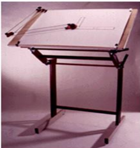
Figure 2. Photograph of a typical college level drawing table, drawing board and mini-drafter assembly
